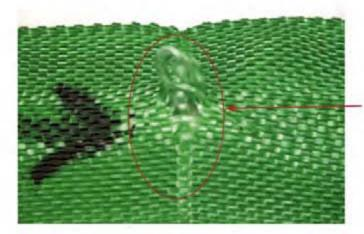
THE DAMAGE: Holes/Snags/Pulls exposing internal core yarns.
